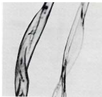
Fig: 1 Microscopic Structure of Cotton
