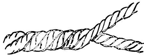
Fig :13 Twist on twist 2 - Ply Yarn
