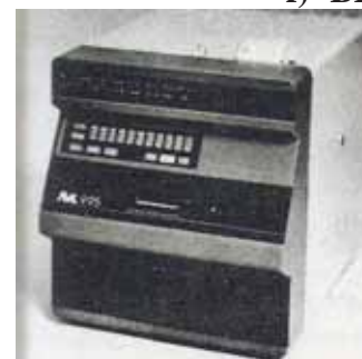
Fig.15-2 Blood gas analyser
